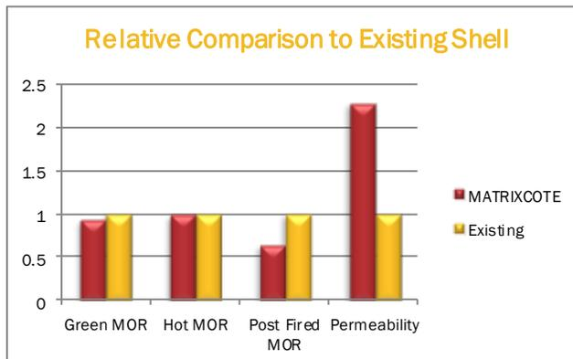
The MATRIXCOTE system tailored to meet the challenge was a combination of Matrixsol® 30 colloidal silica, Matrixcote® concentrate with fiber, and Matrixblend® blue refractory with alumina silicate stuccos. MOR data generated in the laboratory indicated that the MATRIXCOTE system had similar green and hot strength to the existing material. Laboratory data comparing the two shells also indicated that post fired strength was reduced by 35% and permeability was increased by 128%.
