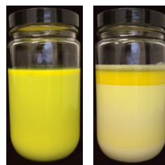
Above left: SUSPENDASLURRY material (after sitting for 3 weeks)
