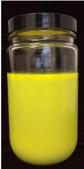
SUSPENDASLURRY material After Sitting For Three Weeks
