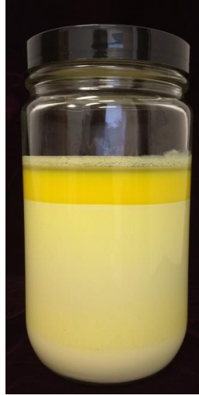
Standard Primary Slurry After Sitting For 24 Hours
