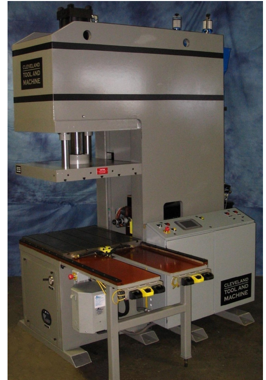
CTM-WI-CF-50 - 50 ton machine with shuttle table and electronic injection control.
