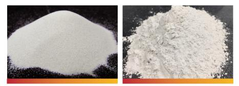
Zircon is almost exclusively used in the primary slurry and as a primary stucco. Because of its high density, zircon provides excellent flow characteristics in a primary slurry. The round grains do not cause defects such as rough casting surfaces.
