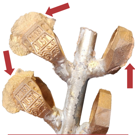
Heavy flashing defect
